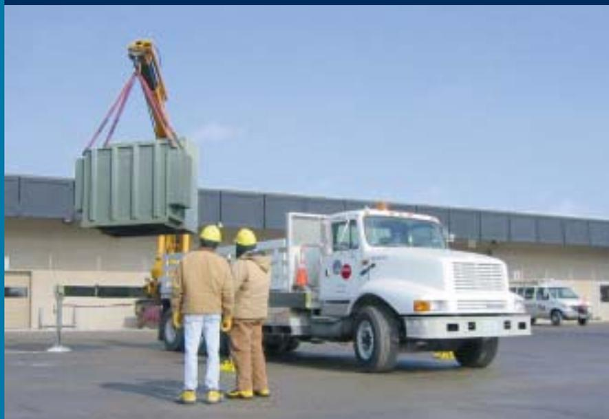
Wisconsin Public Service purchased this heavy-lift knuckle-boom crane primarily for safety reasons. With a lower height, it can lift heavy loads but more easily avoid overhead obstructions. In addition, line electricians can operate the crane by remote control, decreasing any possibility of danger if the crane does touch energized conductors.
